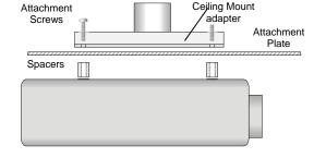
**2.** Position the projector bottom-up. Consult the Attachment Plate Diagram for plate orientation, hole positions and required screws and spacers for your
