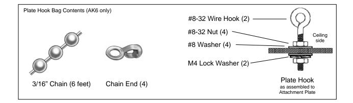
1. Install the Plate Hook Assemblies in the two "H" holes of the Attachment Plate (see diagram) with the hook ends on the ceiling side as shown above. Use pliers to bend the closed hooks apart just enough to install a Chain End at a later time.
