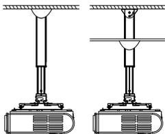
3. The projector mount can also be installed through a false ceiling, (figure 3).
