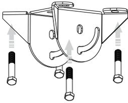
1. Install the Ceiling Mounting Bracket, (figure 1) using the appropriate anchors.
