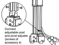
Connect adjustable post and pivot adjuster (screws of accessory 4)
